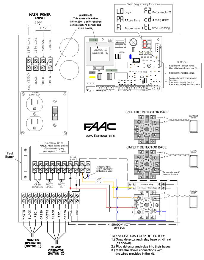
Figure 13. Pre-wired Enclosure with the 455 D Control Panel
