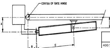
Figure 5. Important mounting dimensions for outward swing 400 operators, top view
