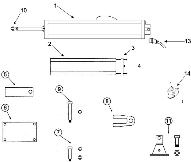
Figure 1. Parts of the 400 Operator
