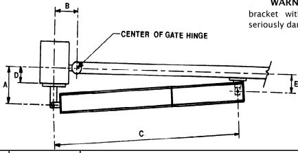
Figure 4. Important mounting dimensions for inward swing 400 operators, top view
